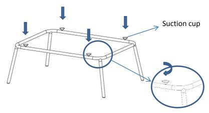
4 Put the table frame upside down onto the table top. The table top is marked where the suction cups should be positioned.
